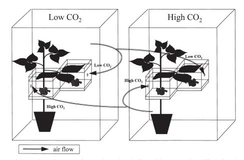
**Figure 1.** Diagram of the experimental apparatus for exposing soybean leaflets to  $CO_2$  concentrations different from those around the rest of the plant.
