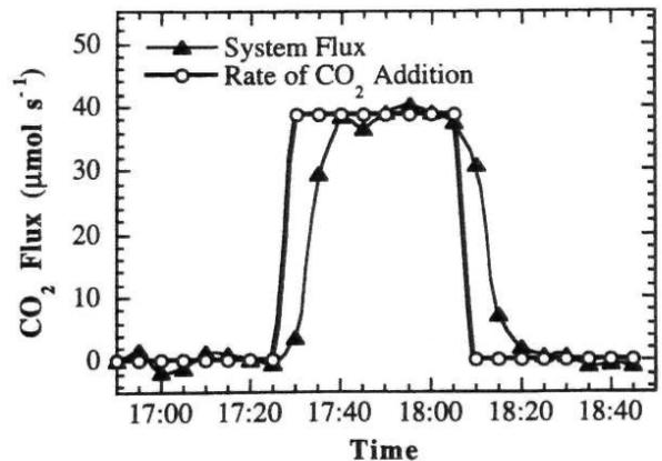
**Figure 2.** CO<sub>2</sub> calibration of EcoCELL precision. A flow of 38.8 μmol s<sup>-1</sup> of CO<sub>2</sub> was added directly to an empty EcoCELL. The calculated flux from the EcoCELL exchange increased by a similar amount. The CO<sub>2</sub> addition and calculated flux lines are slightly offset for illustration; the resulting time constant is <15 min.
