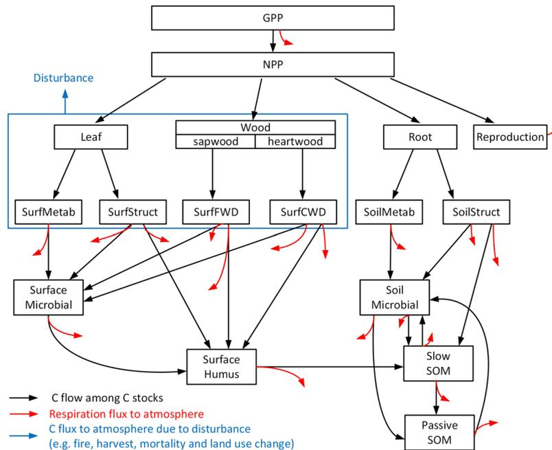
**Figure 1.** Schematic representation of the C transfers among multiple stocks in vegetation and soil (including litter) in LPJ-GUESS. The traceability framework adopts the same structure and preserves all relative flows between C stocks.
