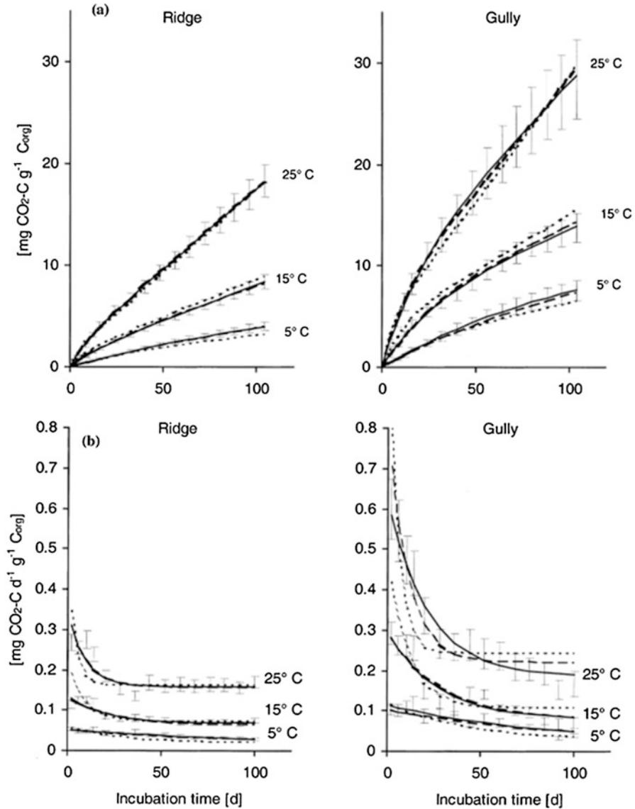
**Fig. 6** Measured and modelled cumulative soil CO<sub>2</sub> emission (a), and soil respiration rates (b) of Gully-Ah- and Ridge-organic-layer soil samples incubated at 5 °C, 15 °C and 25 °C. (Adapted from Reichstein et al. 2000)
