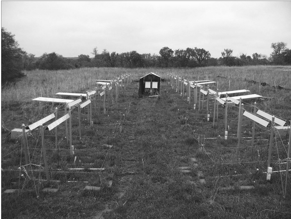
PLATE 1. A 4°C warming experiment by infrared heaters in a tallgrass prairie established in Oklahoma, USA. Photo credit: Y. Luo.
